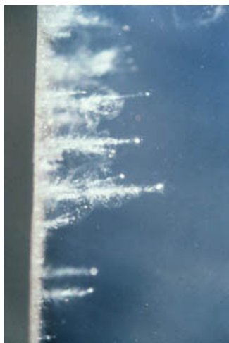
The Stardust spacecraft used a grid holding aerogel to capture dust particles from comet Wild 2. In this test, high velocity dust particles are stopped unharmed at the end of cone shaped tracks in a sample of aerogel
