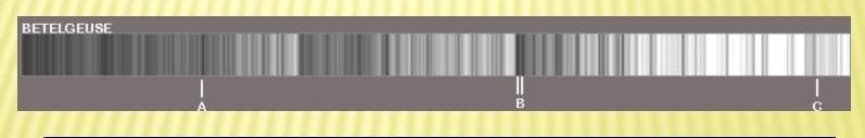
[A] = H-beta line 4861.3 A [B] = Mg line 5167.3 & 5172.7 [C] = Hg emission line 5460.7 A from reference source
