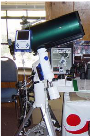
This is the Vixen Sphinx mount with the Star Book controller. The controller features an integrated star map display for controlling the telescope.
